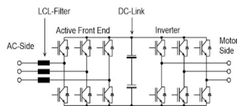
Fig. 1. Active Front End Converter
