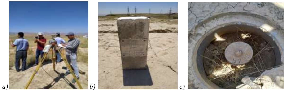
Figure 3. Second geodetic network in Zarmitan area: a- determination of coordinates geodetic network; b- the sign placed on the geodetic network; c- ground repertoire.
