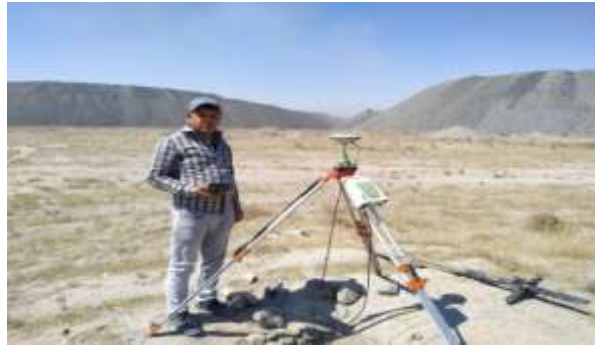
Figure 5. Measurement of the checkpoint at the landfill using GNSS.
