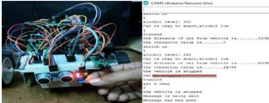
Figure 24 Accident Detection by Sensing Vibrations in the vehicle
