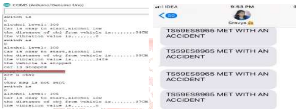
Figure 24 Accident Detection by Sensing Vibrations in the vehicle
