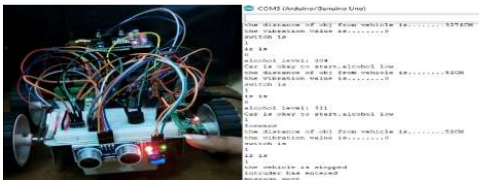
Figure 29 Theft detection by IR sensor detecting 1 Figure 30 message is sent when switch &IR read 1
