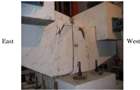
Figure 7 Damage in the irregular beam
