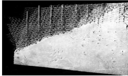
Fig. 3 A Typical Ferro cement Section IV. Construction Methods And Applications:
