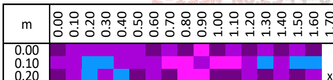
Fig. 19 Corrosion mapping of ground level brace B2 Table 7 Interpretation of corrosion mapping of brace B2
