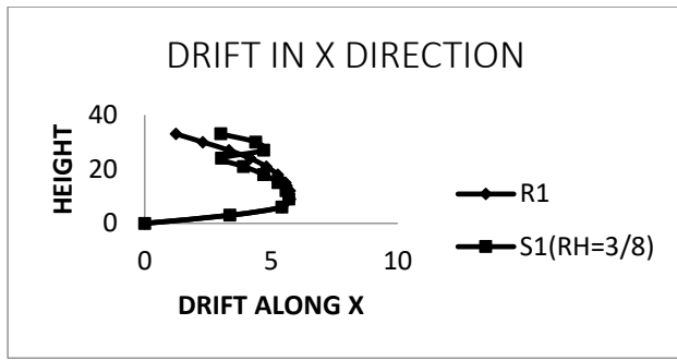
Graph No 9 Graph Showing Storey Drift in X & Z direction for RA=0.25 and RH=3/8
