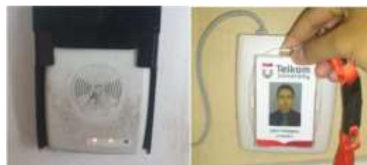
Figure1: Installed RFID Reader
