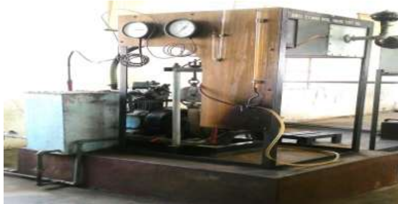
Fig1.7.1: Single cylinder four stroke diesel engine set up
