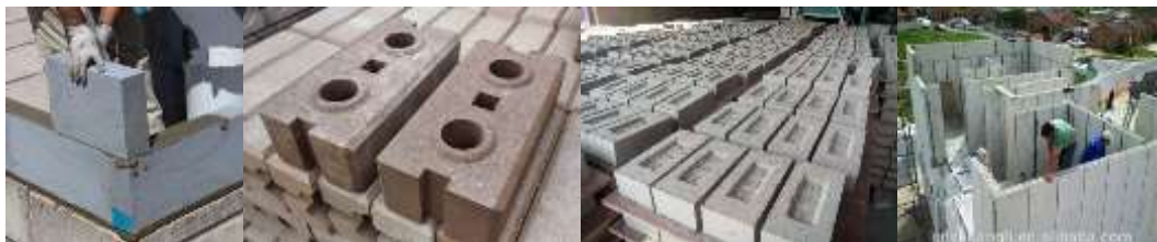
Figure 1. Examples of energy-efficient building structures based on a mixture of coal ash.
