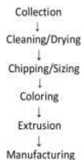
Fig -3: Mechanical recycling process of plastic waste
