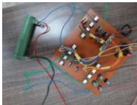
Fig. 4 PCB with connected components and a test load of 500 ohms.
