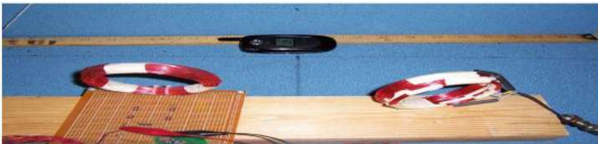
Fig 2.1: Magnetic coupling test set-up
