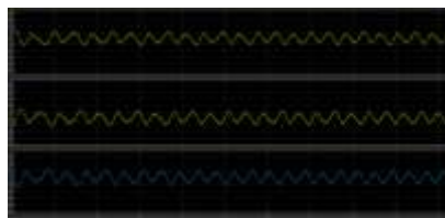
Fig5. Output currents of inverter circuit
