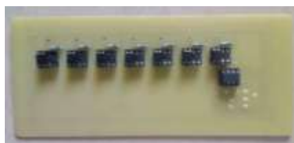
Fig20: PCB Layout of gate driver circuit with components placed
