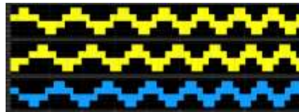
Fig4. Output Voltages of inverter circuit
