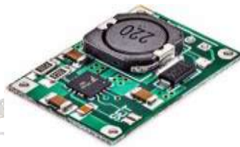
Fig.9 TP5100 Battery Charger
