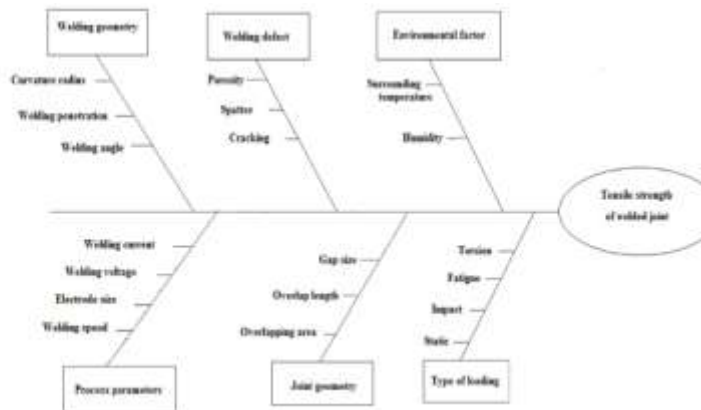
Fig.No.1 Cause and effect diagram of Welded Joint
