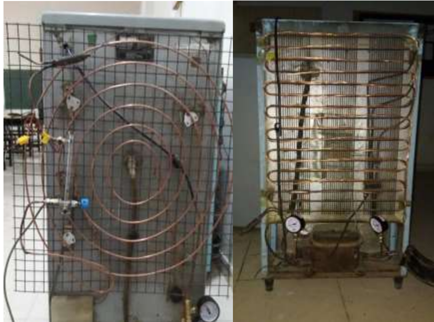
Fig. 3 VCR installed with Spiral condenser and Microchannel condenser
