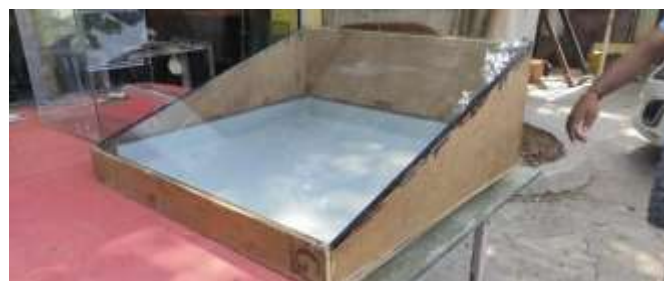
Fig no 3.4.1(6) glass cover of 5mm thickness
