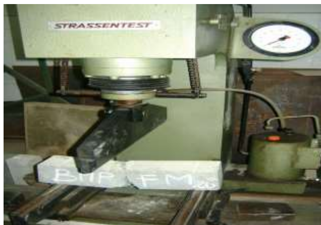
Figure 8: Machine of flexural strength.
