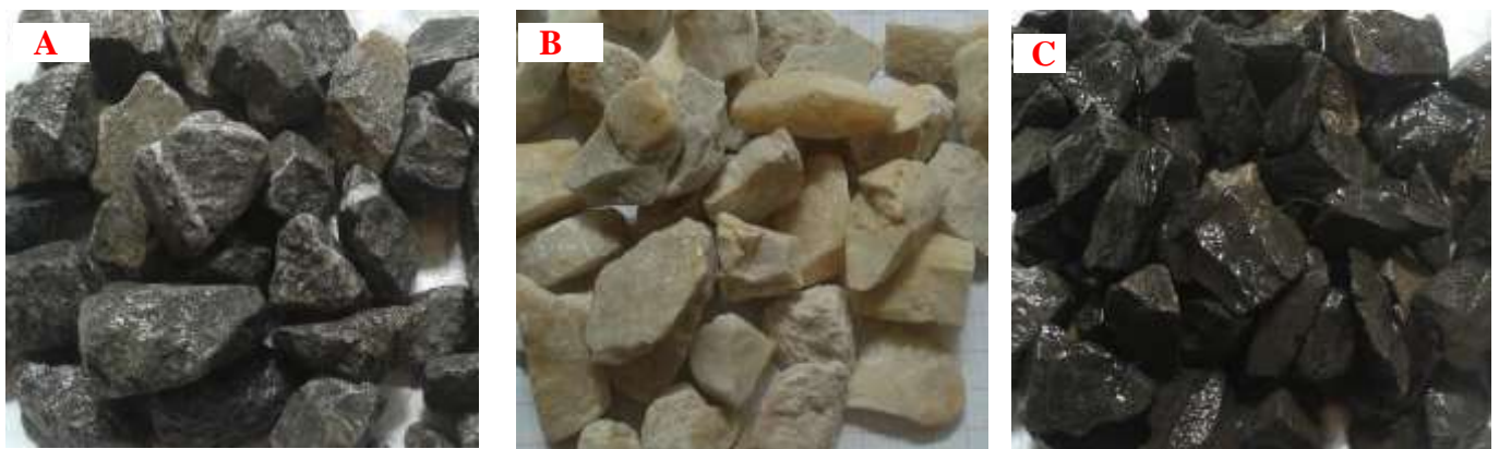
Figure 1: Morphology of aggregates used:A) Crystalline limestone, B) Pure limestone, and C) Marly limestone.
